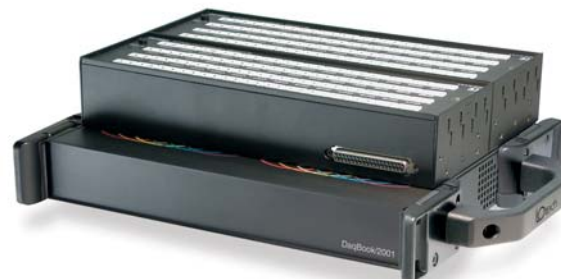
DaqBook/2001 plus 112 channels of thermocouple input (DBK90)
